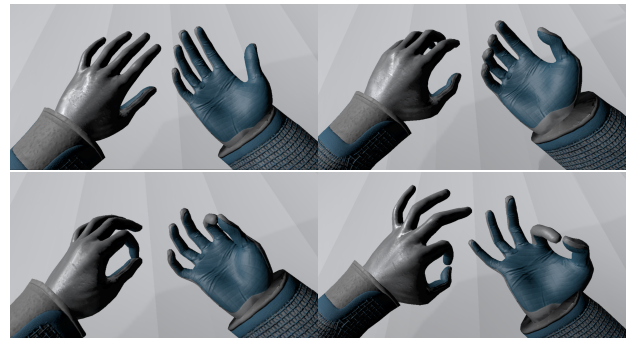
Figure 2: The virtual Astronaut hands. The “relaxed” (top) and “grasping” (bottom) virtual hands as controlled by Hand Tracking (left) and VR Controllers (right). In the Hand Tracking condition the virtual hand follows the users' detailed finger motions, in the VR Controller condition the poses are pre-defined.
