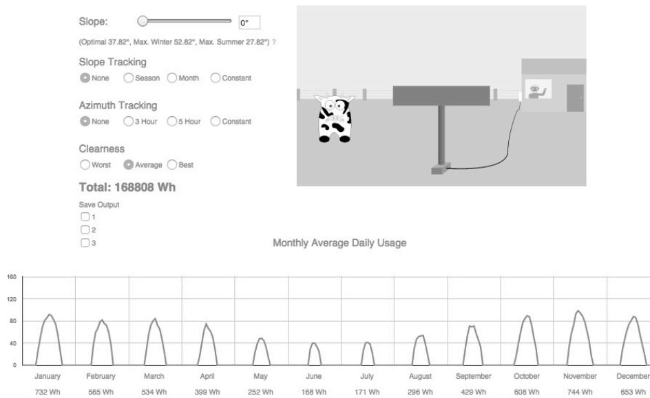
Figure 1: Last page of the tool allows the user to adjust the solar panels orientation, tracking and type of day (worst recorded day, average day and best recorded day). When adjusting these values the power output graph is updated in real time, making it visually noticeable the effects of different configurations.
