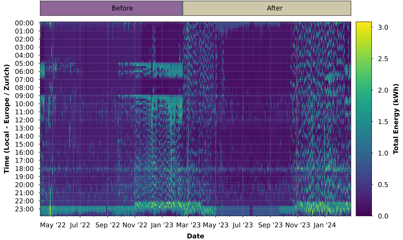
Figure 2: Example of 15-minute resolution SMD for a single household (Household_ID: 461158) visualized as a heat map. The graph shows total active electrical energy consumption (in kWh) using colored pixels, with the date on the x-axis and the time of day on the y-axis. A shift in consumption patterns is noticeable after the energy consultant's visit, where the night setback was deactivated as part of the HP optimization.
