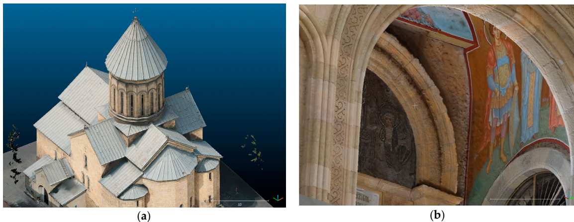
Figure 16. Final 3D model based on combined laser scanning (Faro point cloud) and photogrammetry: (a) 3D view of complete church; (b) detailed view of entrance hall.
