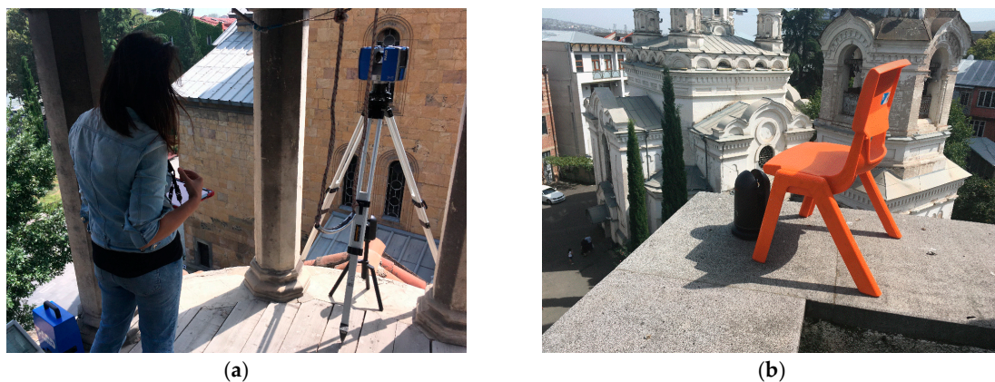
Figure 2. Terrestrial laser scanners: (a) Faro Focus 3D X330 placed on a neighboring bell tower; (b) Leica BLK360 placed on a neighboring roof under a chair for sun protection.
