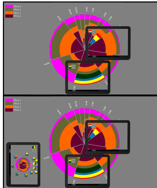
Figure 4. Public time-pie visualization of energy consumption by all the offices in coupled interaction around the tabletop with tablets. The left picture shows details of devices for Office 1 between 8:00 and 10:00, and Office 4 between 12:00 and 14:00. The right picture shows a combination of tablets, each with a different type of details for one of 3 of the offices.
