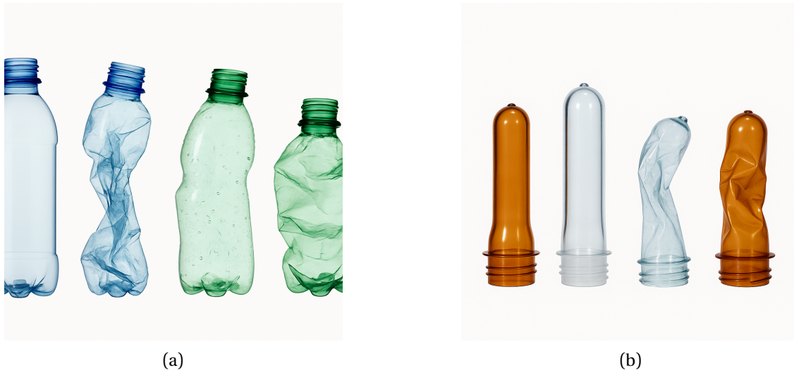
Figure 1: (a) Molded and defective PET bottles; (b) Preforms with different designs.
