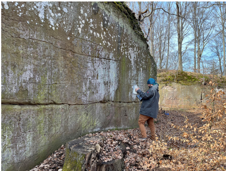
Figure 5. Conducting the 3D scan in the Fingalshöhle with the Artec EVA.
