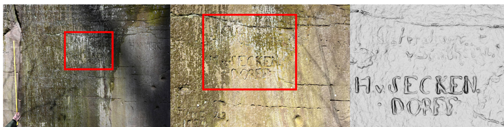
Figure 11. Graffiti mentioning “H. v. Seckendorff” and the more delicately carved “G. Krahiser v. Sontheim” above, unreadable in photographs with different lighting and moisture conditions.
