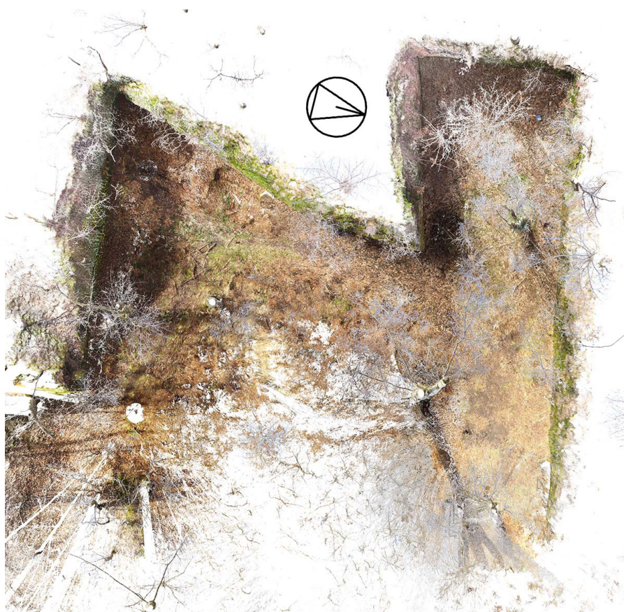
Figure 4. Point cloud overview of the 1225 m 2 area of the abandoned quarry; the point cloud could serve as a basis for a ground floor plan and as a general 3D documentation.
