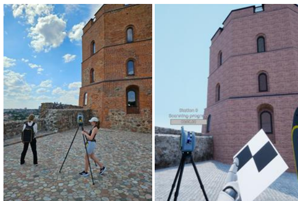
Figure 1. A comparison showing a real-world scanning setup alongside its digital twin equivalent in the VRscan3D simulator.
