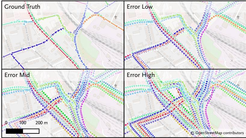
Figure 5.4: Artificial noise error ( E ) scenarios – The top left panel shows the ground truth. The top right panel shows low error noise applied ( E_L ), the bottom left panel shows middle error noise applied ( E_M ), and the bottom right panel shows high error noise applied ( E_H ).
