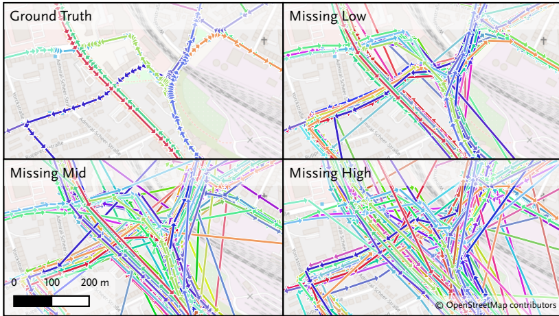
Figure 5.7: Artificial missing points error ( M ) scenarios – The top left panel shows the ground truth. The top right panel shows few missing points applied ( M_L ), the bottom left panel shows average missing points applied ( M_M ), and the bottom right panel shows many missing points applied ( M_H ).
