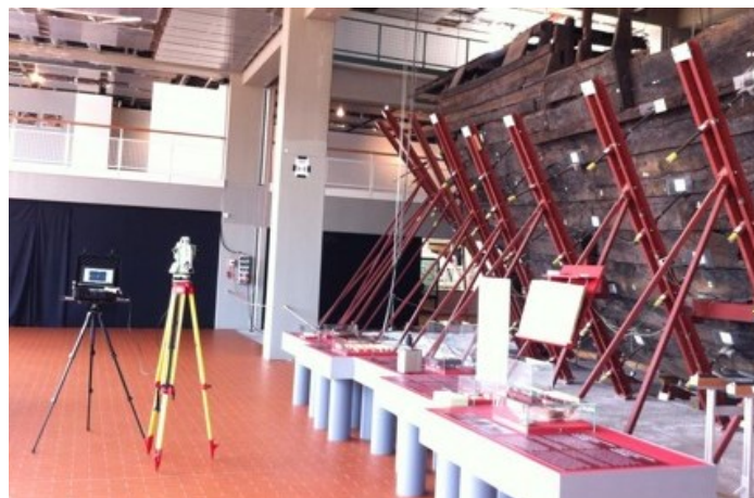
Figure 12-6: Example of the working set-up. The total station connected to the portable PC (Ditta 2015).
