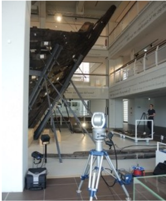
Figure 4-8 : Laser Tracker in front of the Bremen Cog, DSM, Bremerhaven (A. Colson 2017)
