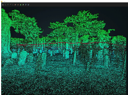
Figure 3. Image of 3D mobile laser scanning in operation, Jewish Cemetery Walsdorf in Franconia, Germany.
