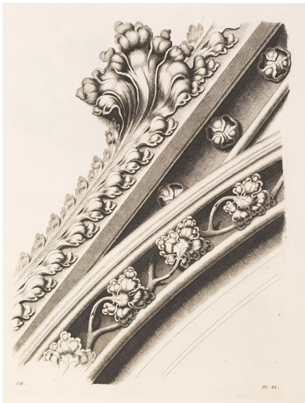
Ill. 10 Detail of the junction of the over-arch and gable on the west portal of York Minster, from Halfpenny 1795, pl.41
