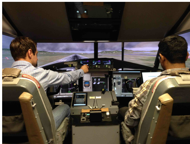
Figure 3. Current simulator cab with lab-designed Prototype Design. Participant sits at left (Captain’s seat) and experimenter at right (First Officer seat). Experimenter uses tablet computer to control progress through the experiment.
