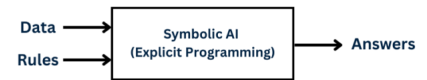
Figure 2.1: Schematic representation of symbolic AI: explicit programming combines data and rules to produce answers (Adapted from: Fig. 2, https://machinemindscape.com/artificial-intelligence-to-deep-learning-history-concepts/ ).
