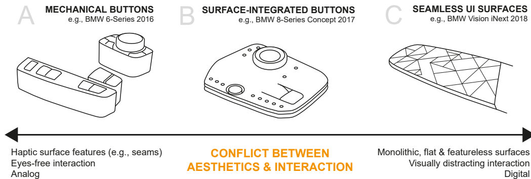
Fig. 2.: The surface-integration of in-car control elements, such as buttons and rotary dials, creates a conflict between aesthetics and interaction.
