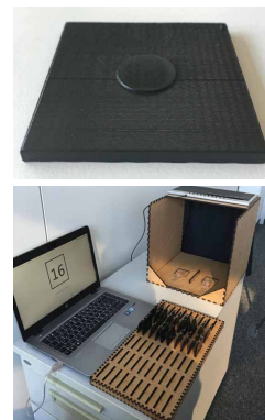
Fig. 1. The experimental stimuli were made from laser-cut polycarbonate and presented blindfolded in a touchbox. The MDS configuration shows four clusters with their corresponding shapes and ID. The white color depicts protruded areas in the tactile plates.
