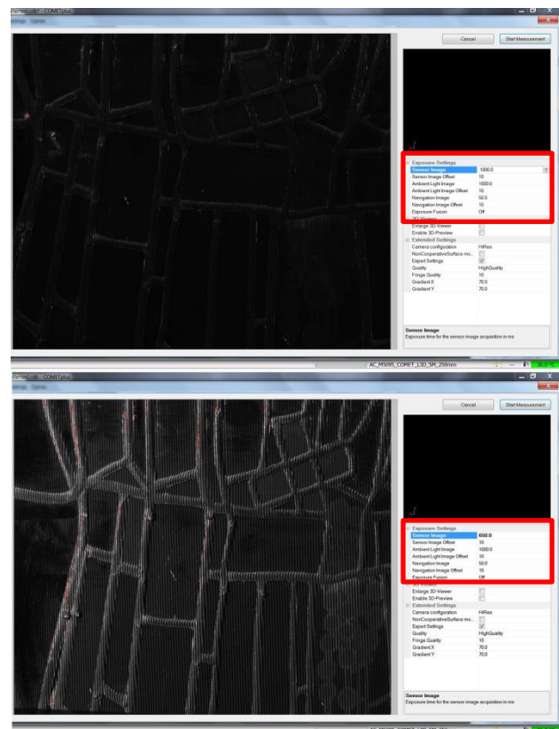
Figure 2. Oswiecim 2b; Comparison of different light setups, within the scanner software, with and without the use of polarising filters. Upper part: Setup with filter; highest possible light settings don't provide enough light for scanning. Lower part: without filter, but scanner located 70° to surface; ideal light settings.
