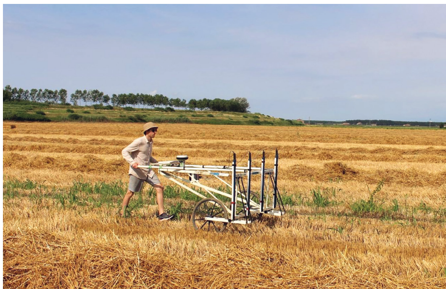
Figure 3. Magnetometer survey in July 2023, using a LEA Mini system with four SENSYS FM650 probes and a Leica GS15 GNSS antenna mounted on the cart. In the background the dike of the Po di Goro is visible (photo W. de Neef).
