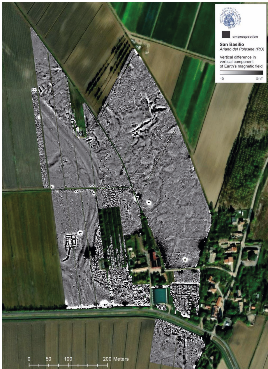
Figure 4. Overview of the results of the magnetic gradiometry surveys. Dynamic range \pm 5 nT.
