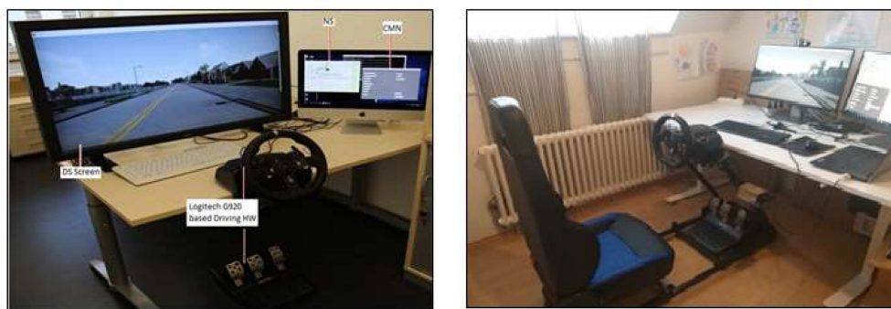
Figure 2: Minimal BeaCON setup without driving seat (left), BeaCON setup with driving seat for enhanced user experience (right).
