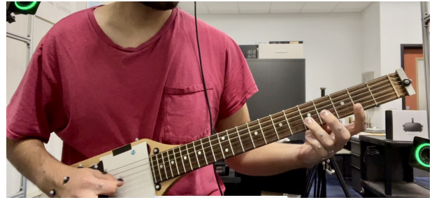
Figure 4: The motion capture setup. Small markers are placed on the musicians hands and around the guitar and are tracked with 15 OptiTrack cameras at 120 frames per second.
