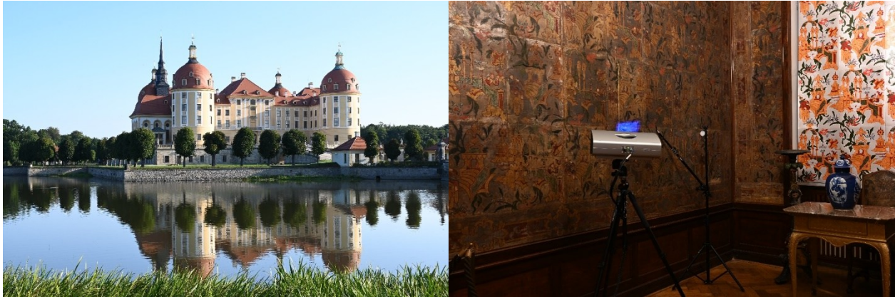
Fig. 1. Left: Castle Moritzburg from the 18 th century is situated in Saxony 15 km north of Dresden. Right: The Chinese Room inside the castle is an example of one of 11 rooms showing original leather panels. The examination of the historic surface was conducted by structured light scanner combined with precise microclimate monitoring (© Kristina Holl).
