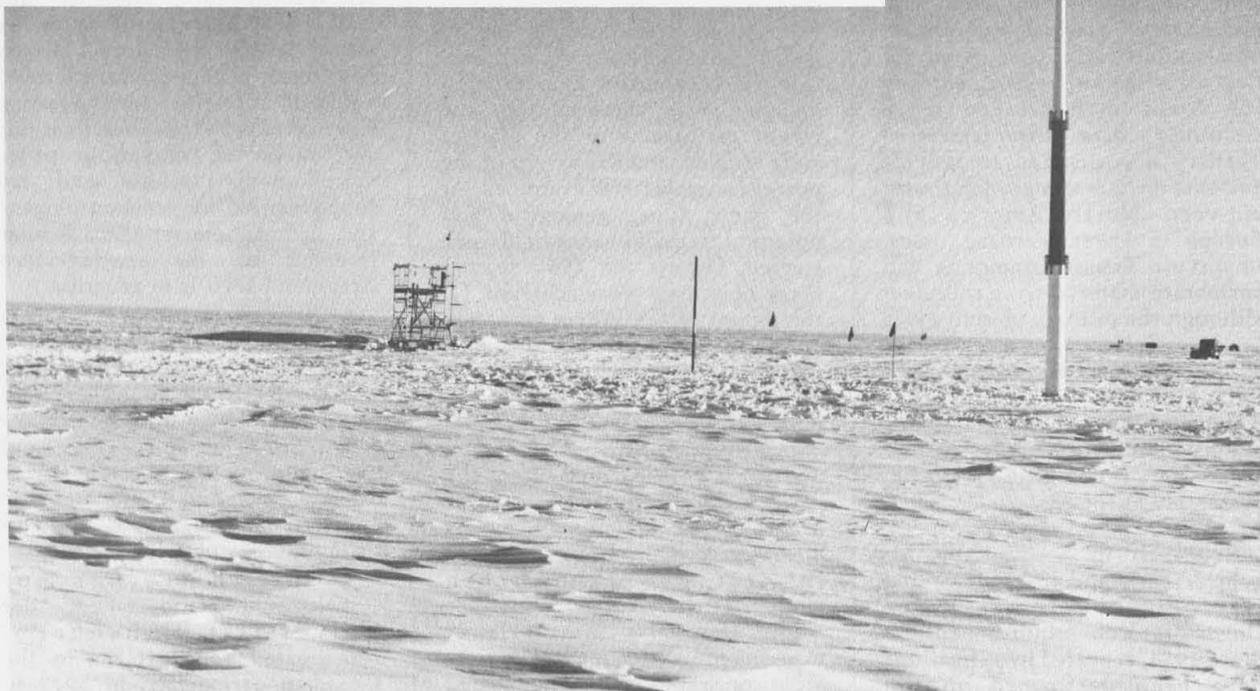
Figure 1. This is one of the 18m glaciological and geodetic markers (Haefeli-Balise) planted on the EGIG traverse profile for long-term observations. The geodetic survey tower and accumulation stake are to the left.
