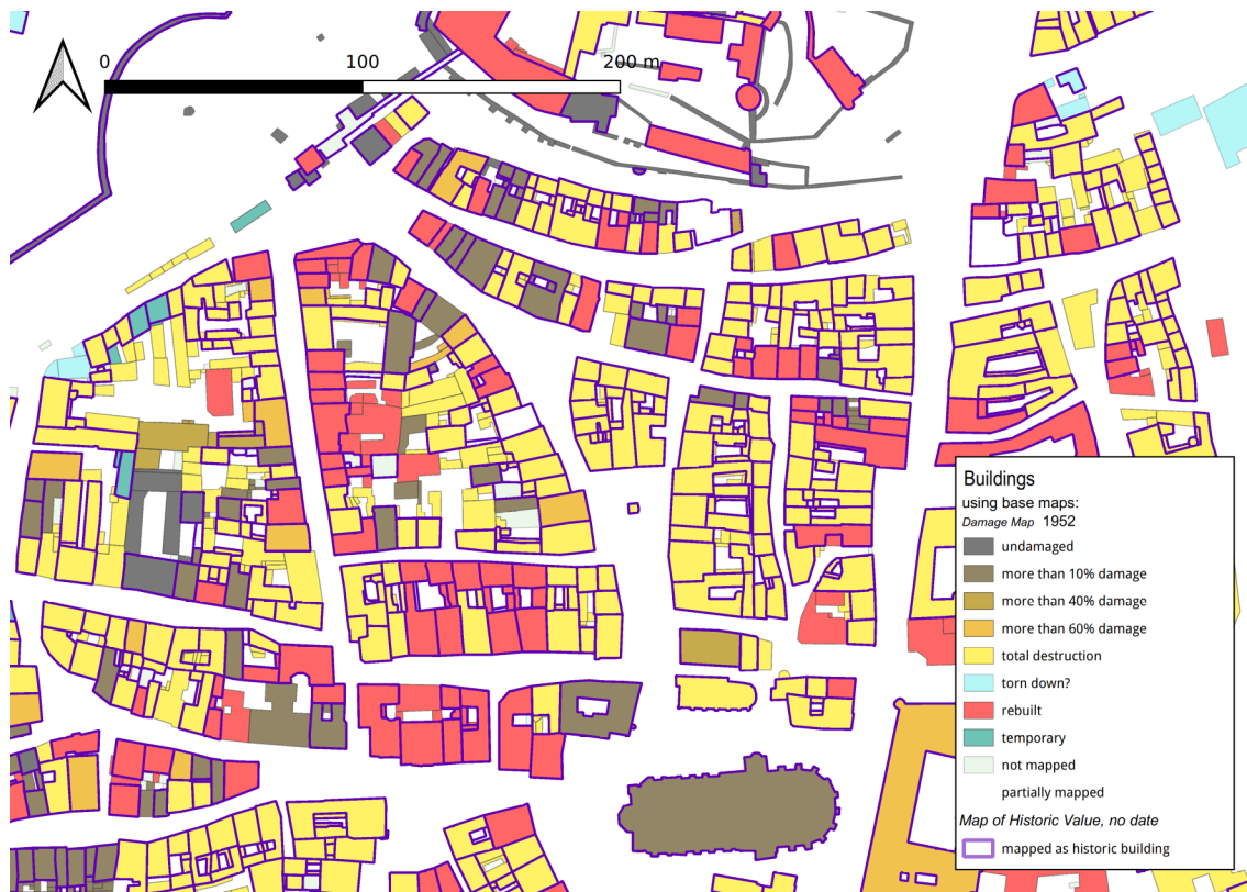
Crop of a multilayered GIS map showing the relation between the degree of destruction and historic value as taken from the Damage Map 1952 (StadtAN_A4_X_265) and the Map of Historic Value, no date (StadtAN_A4_X_210).
