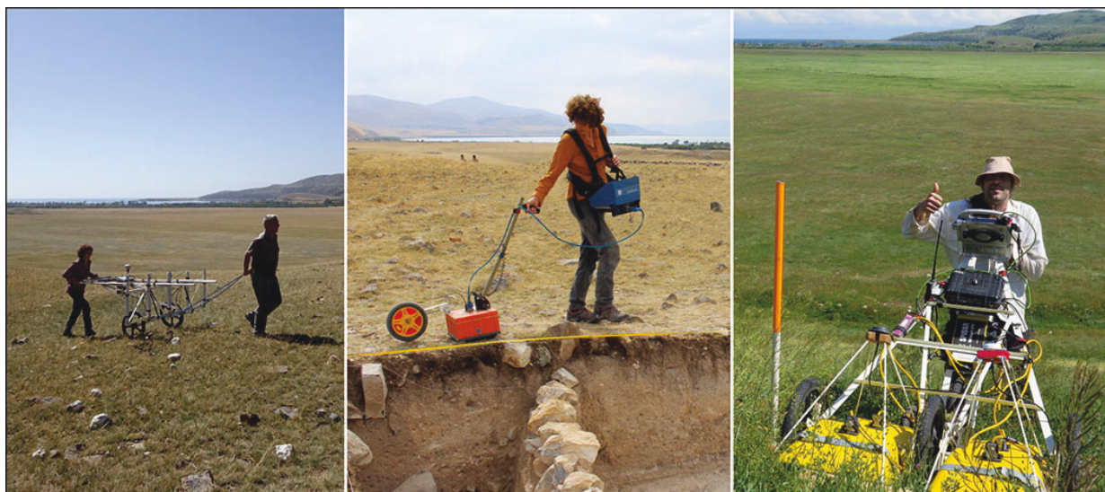
Figure 4. Geophysical methods in use at Artanish 9; left) magnetic gradiometry (2022); centre) GPR (GSSI SIR with single 400MHz antenna, 2022 & 2024); right) GPR (PulseEko Spidar bistatic system with two 250MHz antennas, 2023) (figure by B. Ullrich).
