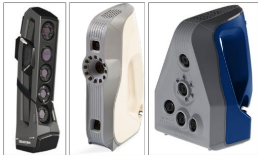
Figure 1: Used and investigated hand-held 3D scanning systems. Creaform GO!Scan Spark (left), Artec EVA (centre), Artec Spider (right).
