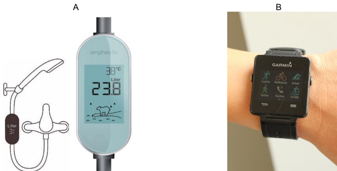
Figure 6. Smart Water Meter for Self-Tracking Water Consumption while Showering (A) – Garmin Activity Tracker (B)
