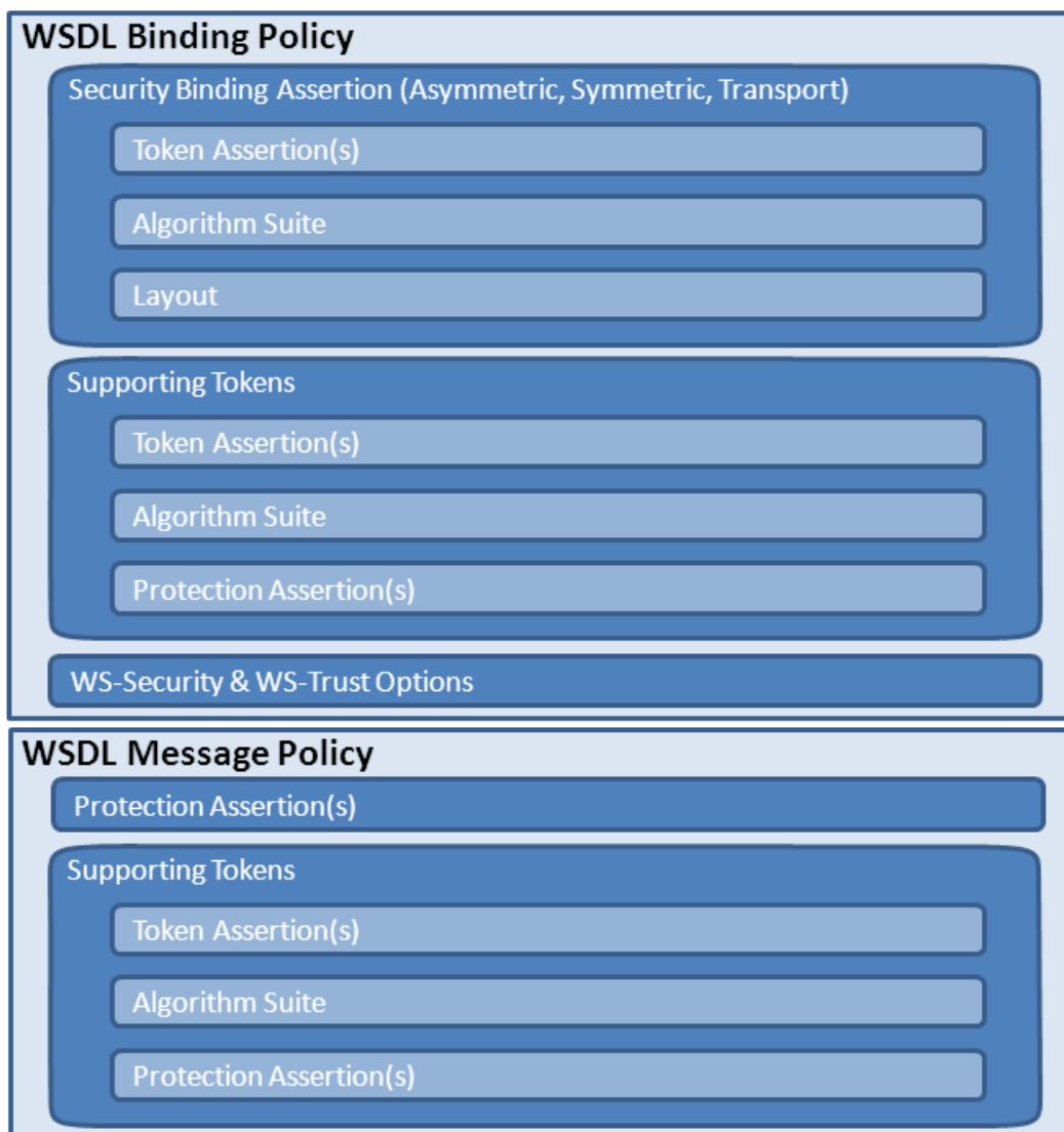
Figure 6: WS-SecurityPolicy elements and structure inside a WSDL document
