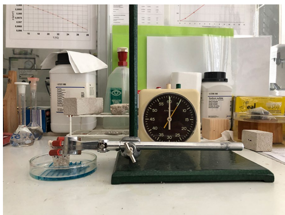
Fig. 12 Measurements of Water Capillary Uptake on a sample of intonaco render layer, according to DIN EN 52617
