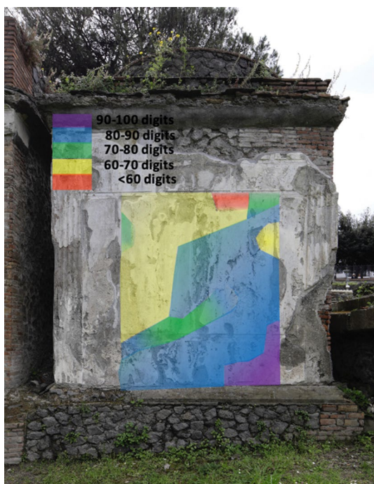
Fig. 16 Tomb PN-EN14, south facade. Survey of moisture distribution using the device Gann Hydromette Compact B. Each range of value (in digits) corresponds to a color (see legend)
