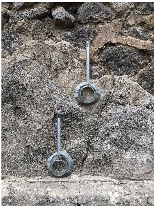
Fig. 8 Measurements of Water Capillary Uptake using Karsten Tubes in the arriccio 0 and arriccio 1 render layers
