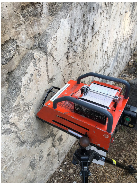
Fig. 15 Tomb EN14, south facade. Area of sampling of powder material and of drilling resistance measurement using the apparatus DURABO®
