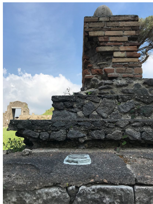
Fig. 9 Tomb PN-EN02. Measurements of Water Capillary Uptake using basin method in the cocciopesto protective layer
